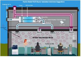
The PurAire SG-FCU/3 Bipolar Ionization unit is designed to be placed inside or mounted in the supply duct or FCU of a ventilation system. The airflow over the dual ionization tubes produces powerful bipolar oxygen ions that flow into the room and saturate the indoor space with the ions.
