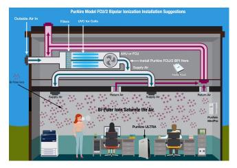
The PurAire SG-FCU/2 Bipolar Ionization unit is designed to be placed inside or mounted in the supply duct or FCU of a ventilation system. The airflow over the dual ionization tubes produces powerful bipolar oxygen ions that flow into the room and saturate the indoor space with the ions.
